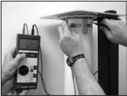
Bottom load collector: testing resistance between cage and tubesheet.
