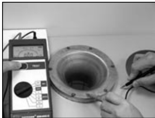
Top load collector: testing resistance between cage and tubesheet.
